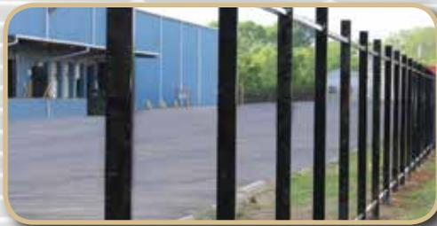
INFINI-RAIL is AMICO's continuous rail design which eliminates cutting rails between posts which is necessary when installing most traditional fences. The AMICO roll formed design has a highly engineered shape and is stronger and lighter than traditional rails. INFINI-RAIL ties the entire system together stretching the full length of the fence. It can also be utilized to run impact and fiber optic cables throughout the fence.
